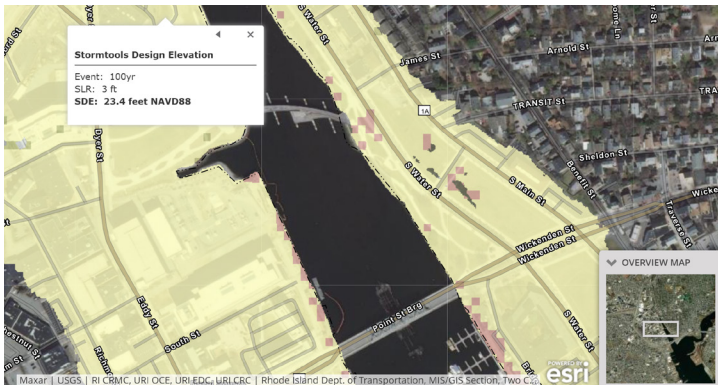
STORMTOOLS inundation mapping for 3' SLR and 100yr storm.
